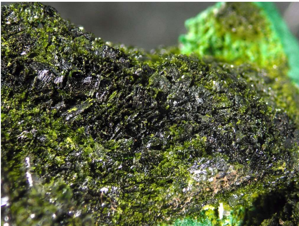
Volborthite from Milpillas mine. FOV of all pictures: 1.2 cm.
