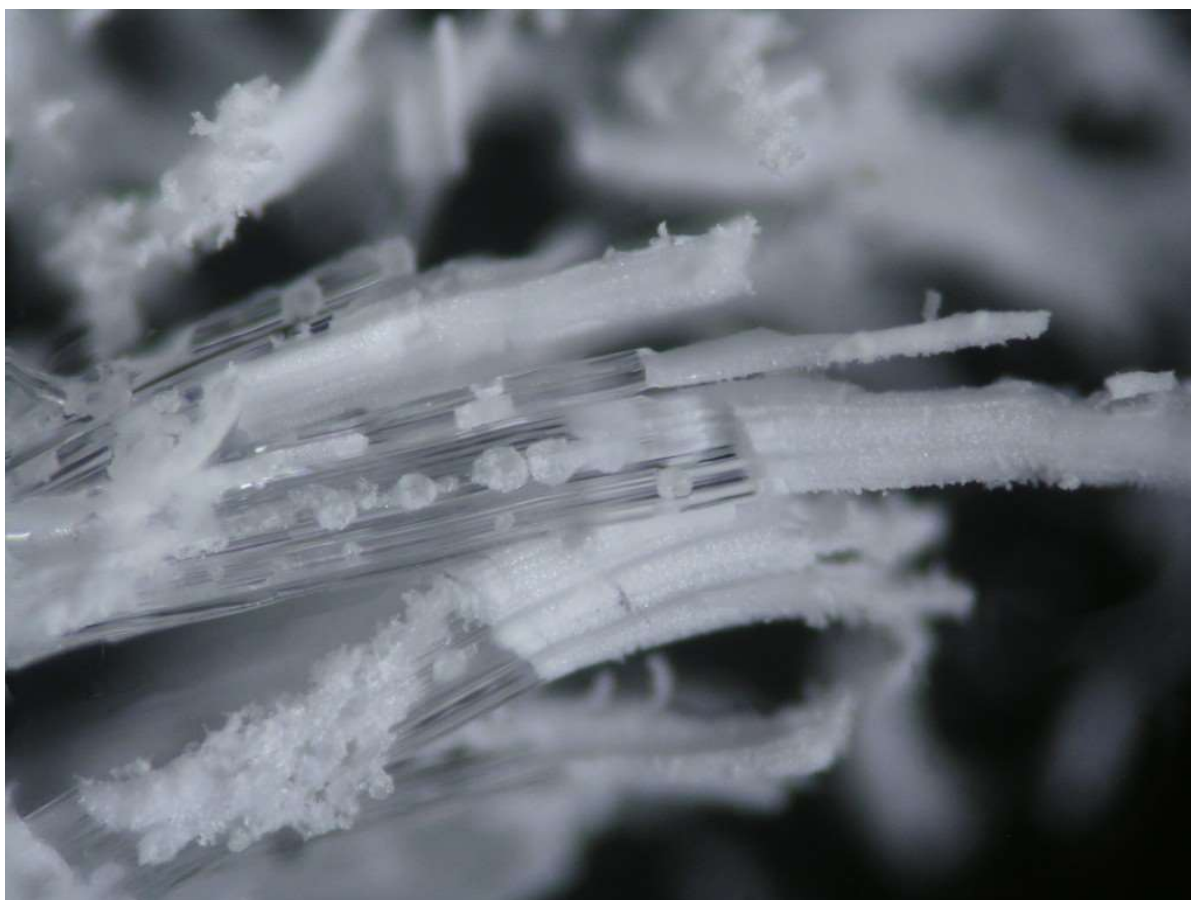
Partially dehydrated epsomite, forming pentahydrate (white)
